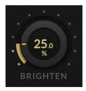
The brighten control is inspired by a common mixing workflow that is often used in conjunction with de-essing: accentuating the high-frequencies in conjunction with deessing to avoid the signal from becoming 'dull'.
