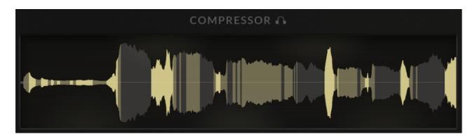
The compression history graph plots the input signal (pre-filter) and highlights parts of the signal that are being compressed.
