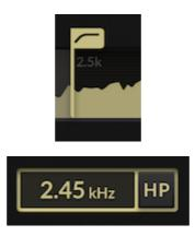
The sidechain filters can be used to remove low or high frequency content from the signal that is triggering the de-esser.
