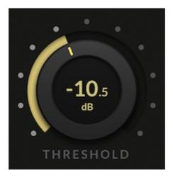
You can set the threshold by dragging the 'THRESHOLD' control, or adding a value directly.
