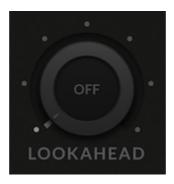
Setting a lookahead allows the de-esser to react to sibilant events slightly ahead of when they occur. Turning the LOOKAHEAD on will introduce latency to the plug-in!
